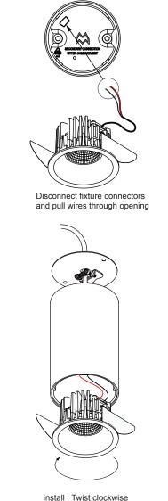
uninstall : Twist clockwise uninstall : Twist counterclockwise
