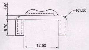
NOTE :-Part :- Small Clamp For Rail Material :- M.S. Plating :- Zinc Plated Assm. Qty - 4 Pcs. Drawing No. :- D-001/e Tolerance :- ±0.10 Scale :- 1.5:1 All dimensions are in mm.
