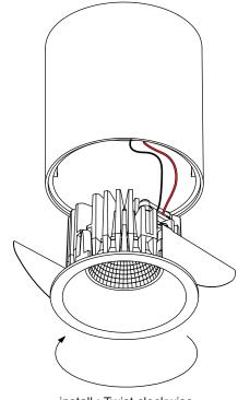
install : Twist clockwise uninstall : Twist counterclockwise
