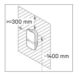
**Attention:** The wall must have a flat structure and must be able to hold a sufficient load. This installation procedure is meant for a concrete or brick wall. If another mounting surface is used, ensure that appropriate screws and/or plugs are used.
