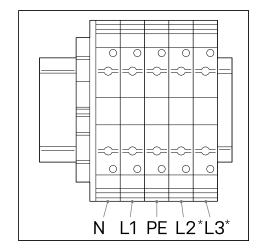
**Attention:** Do not connect the phase cables L1, L2 or L3 in the PE or N connectors.
