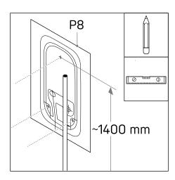
Mark and strip the mains cable at 10mm above the mains wire entrance as indicated on the template.
