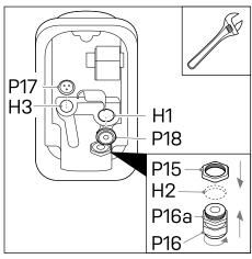
**Attention:** Ensure that grommets and the cable gland are inserted correctly, to guarantee resistance to ingress of water and dust.
