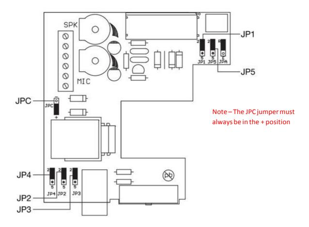
If the 2-wire handset you are replacing has AC buzzer call then the **JPA** jumper must be in the **R** position. If the handset has electronic call the **JPA** jumper must be in the **E** position.
