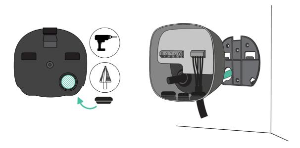
Fix your charger to the wall plate and then fix it using the appropriate screws.
