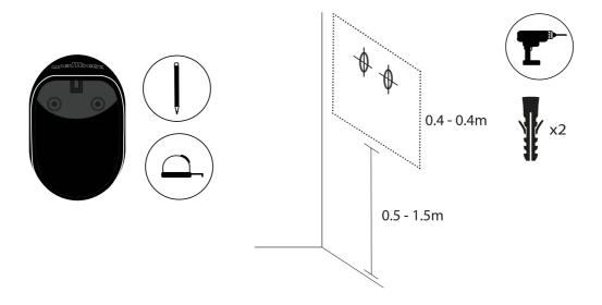
Insert the anchor screws into the fixing holes. Then secure the device to the walls by inserting and tightening the screws.
