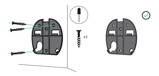
1 If case power supply wiring comes from the wall, ensure to place the wires through the wall plate hole before fixing the wall plate.
