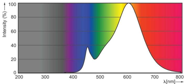
Spectral Power Distribution Colour - Corepro LEDspot 2.7-25W GU10 827
