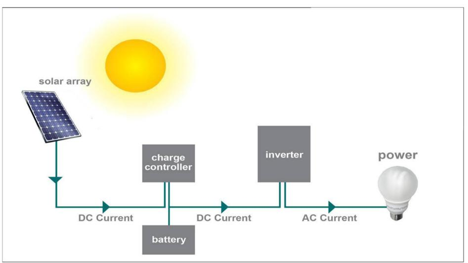
Once solar energy is converted into AC power, it is possible to use this energy to power your appliance, home or even business. If you have an off-grid solar system, then your system will have a rechargeable battery in the loop, right after the inverter. This battery is charged by your solar cells and stores any excess energy, which guarantees that you will always be using the energy you generate yourself, and that you'll always have energy as long as you produce sufficient amounts.
