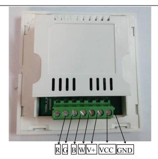
4.1 GND: Cathode of supply power
