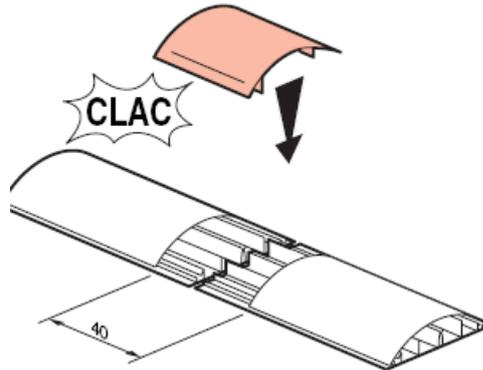
For mounting with floor ducts 92x20mm
