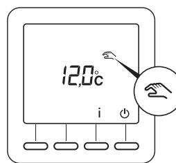
During the external override, if the symbol
