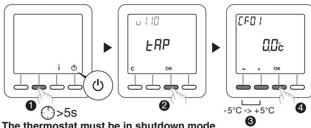
The thermostat must be in shutdown mode.
