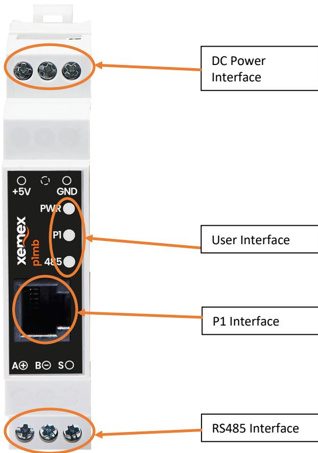
The P1MB is connected via an RJ12 connection to the P1 port of a smart meter. The device is powered by the +5V of the P1 port of the connected smart meter. If not available the P1MB can optionally be powered by an external adapter connected to the DC power interface.
