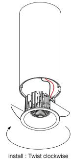
install : Twist clockwise uninstall : Twist counterclockwise
