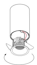
install : Twist clockwise uninstall : Twist counterclockwise
